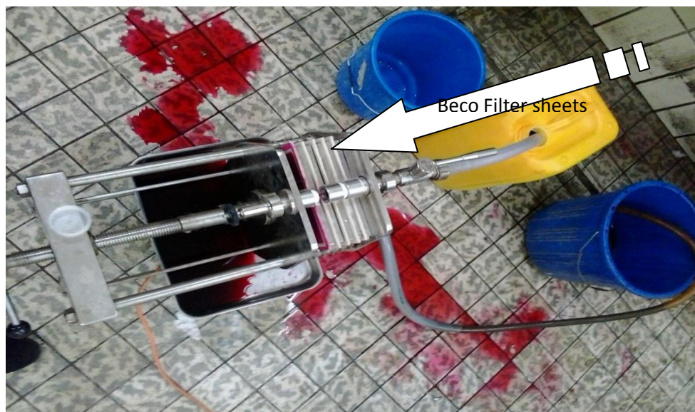
Figure 3-3: Filter press set up
