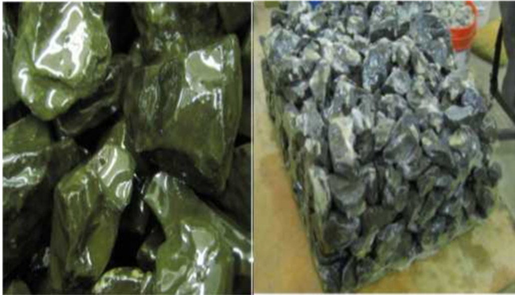
Figure 11: A close view of ELASTOTRACK coated ballast aggregates
