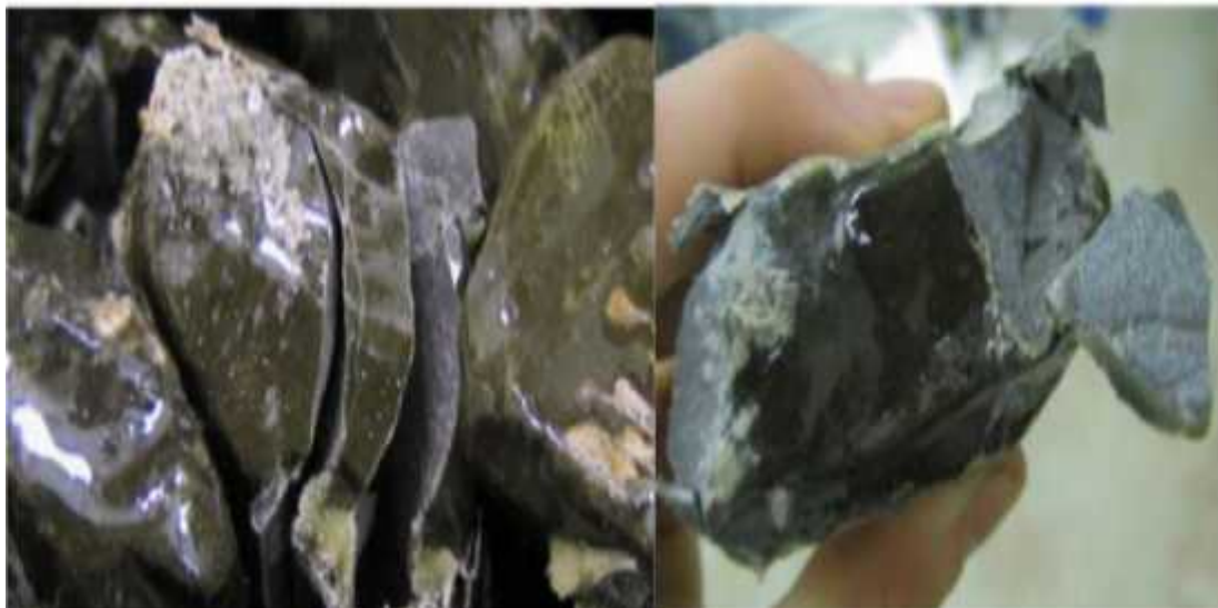
Figure 12 ELASTOTRACK coated ballast aggregates stay intact even after breakage.
