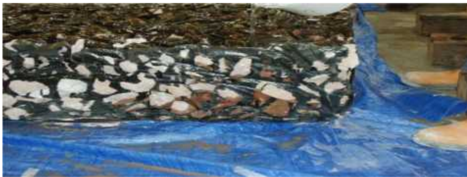
Figure 8 XiTRACK sample still free draining after 200,000 load Cycles
