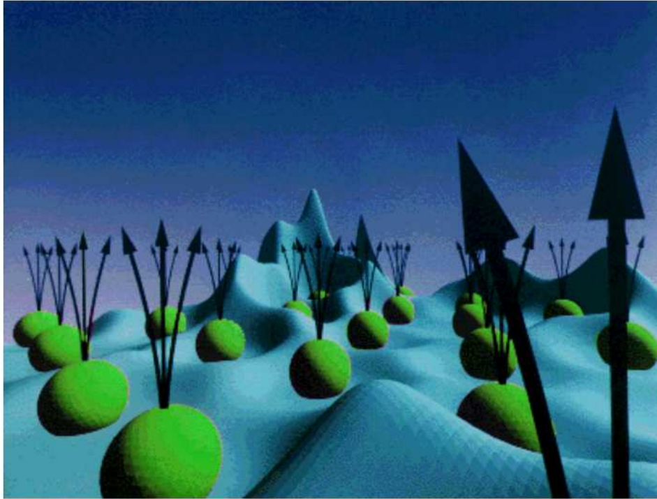
Figure 5.2: Charge distribution of a prototype electron for the \nu = \frac{1}{3} Laughlin wave function. The green spheres represent electrons, while the black arrows represent flux quanta.
