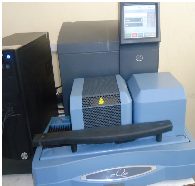
SDT Q600 Thermogravimetric analysis
