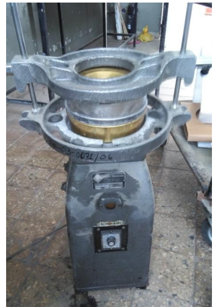
Analytical balance, sieves of different size openings with pan and mechanical shaker for determination of particle size
