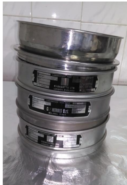
Analytical balance, sieves of different size openings with pan and mechanical shaker for determination of particle size
