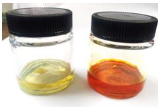
Figure 36 Dip the TiO 2 electrode into the dye solution.
