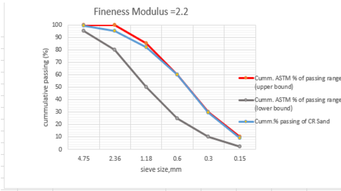
Figure 3.1 Graph for grain size distribution of CR sand for F.M of 2.2
