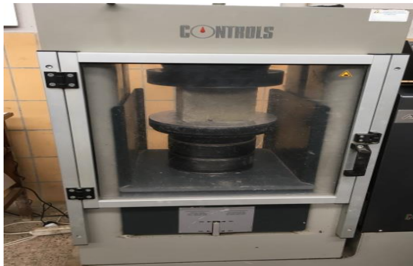
Figure 4.1 Compressive strength of concrete being tested
