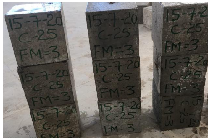
Photo 4. Cube specimens prepared
