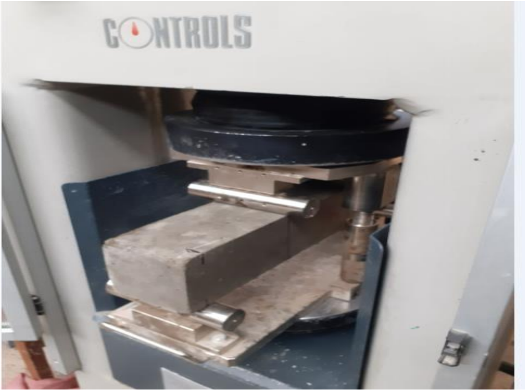
Figure 4.3 Specimen to be tested for flexure
