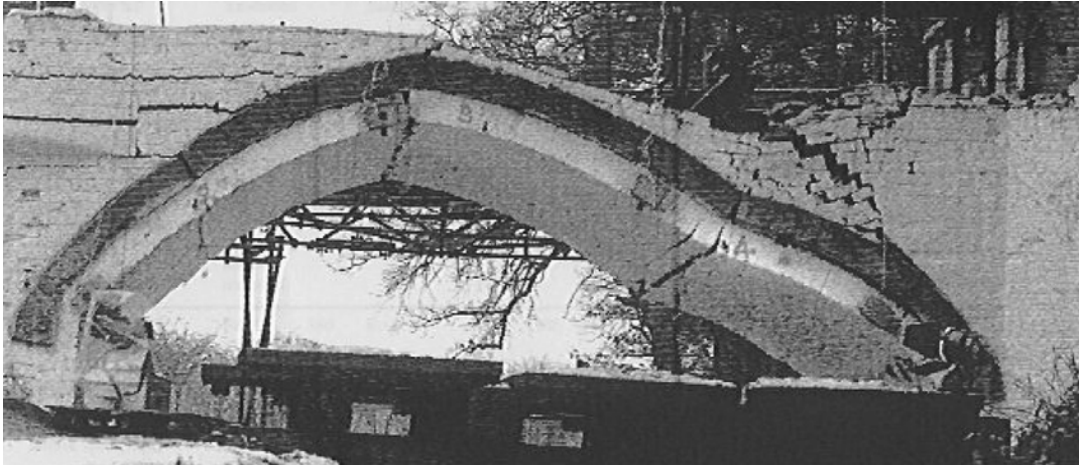
Figure 5-4 Prestwood Bridge: Mechanism (Page,1987)
