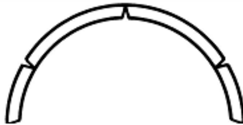
Figure 2-6 Collapse Mechanism of an Arch (Heyman J.)
