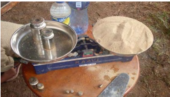
Photo-3 Measuring of soil samples for blending.
