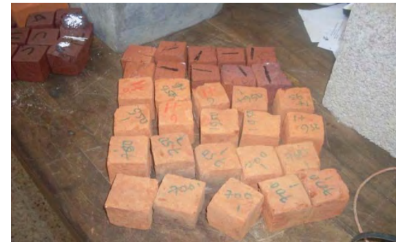
Photo-7 Fired clay bricks produced blended soil sample B-2.
