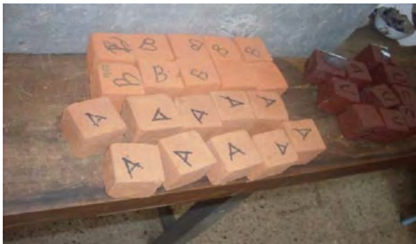
Photo-6 Fired clay bricks produced from the blended soil sample B-1.
