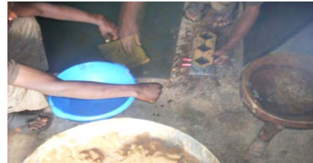
Photo-4 Painting the form works with food oil during shaping stage of brick production.
