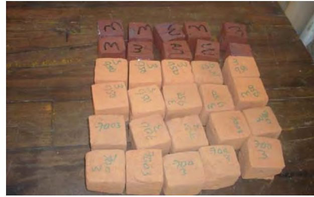
Photo-9 Fired clay bricks produced from the blended soil sample B-4.
