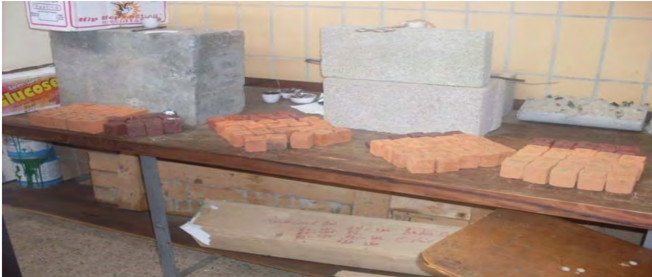
Photo-5 Fired clay bricks produced from the four blended soil samples.
