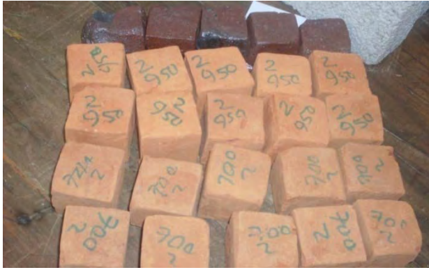
Photo-8 Fired clay bricks produced from the blended soil sample B-3.
