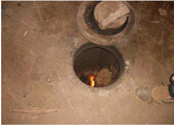
Photo-12 Inspection hole for controlling the degree of firing of bricks in Burayu brick factory kiln.
