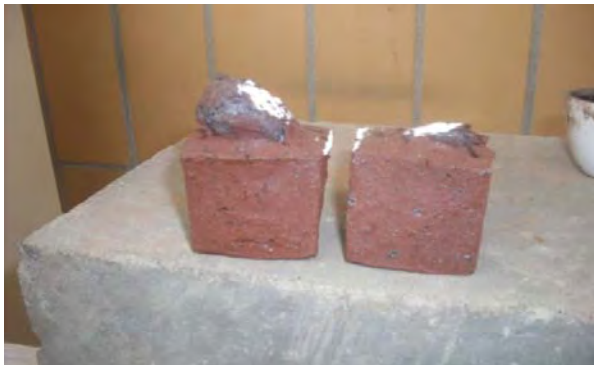
Photo-10 Fired clay bricks produced from the blended soil sample B-1 which starts melting at a firing temperature of 1200°C.
