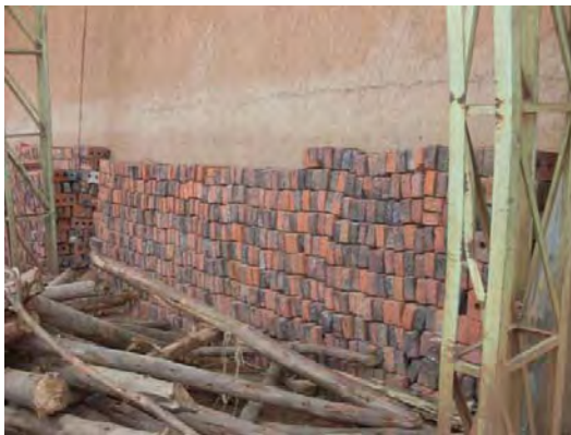
Photo-14 Over burnt bricks in Burayu brick factory.
