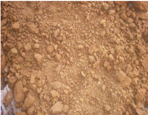
Photo- 1 Drying of red clay soil in the brick production site.
