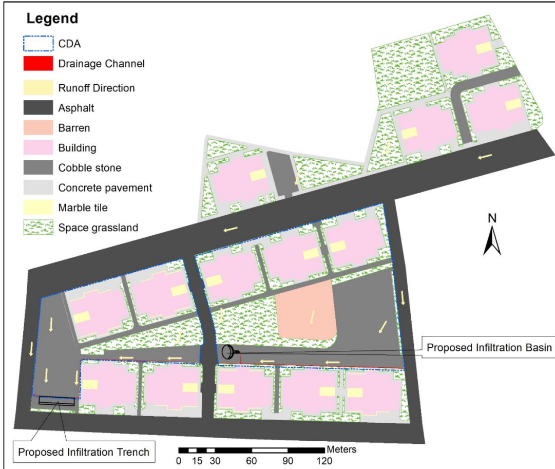
14Figure 4.5 Proposed Infiltration trench and basin
