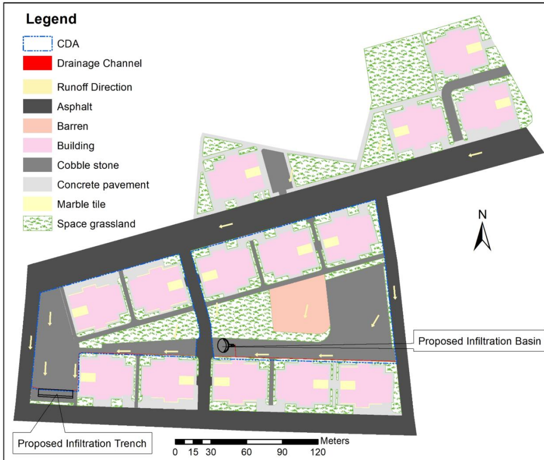
Figure 4.1 Proposed Infiltration trench and basin
