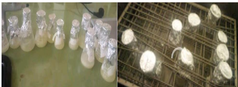
Annex 5: Lipase production test on 1% v/v butter fat supplemented nutrient agar
