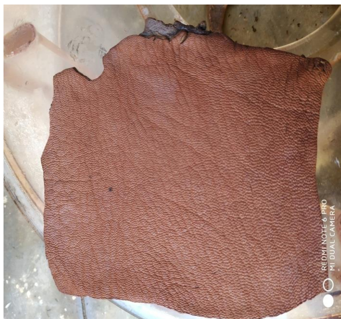
Figure 4. 19 Leather sample re-tanned with enzyme pretreated powder
