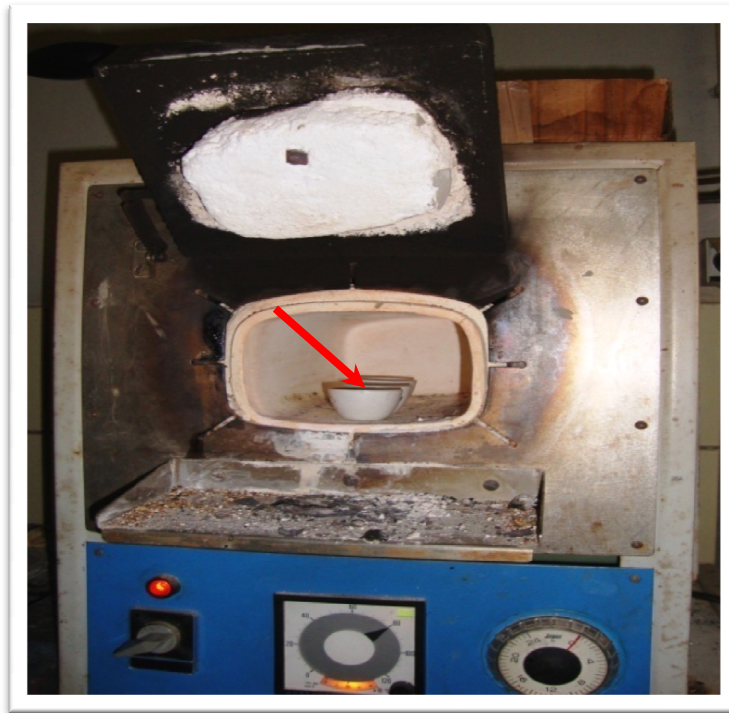
Figure 3.4. Ash content analysis in muffle Furnace. Arrow points to the sample
