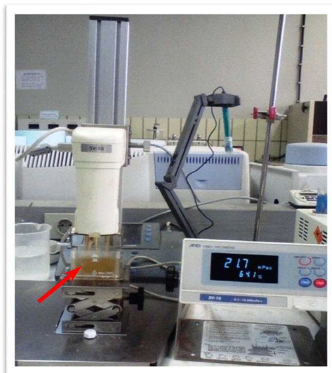
Figure 3.2. Samples in the viscometer for viscosity measurement. Arrow points to the container with the sample solution
