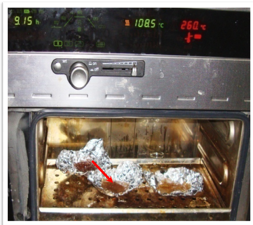
Figure 3.3. Sample in the oven for moisture content determination. Arrow points to the sample
