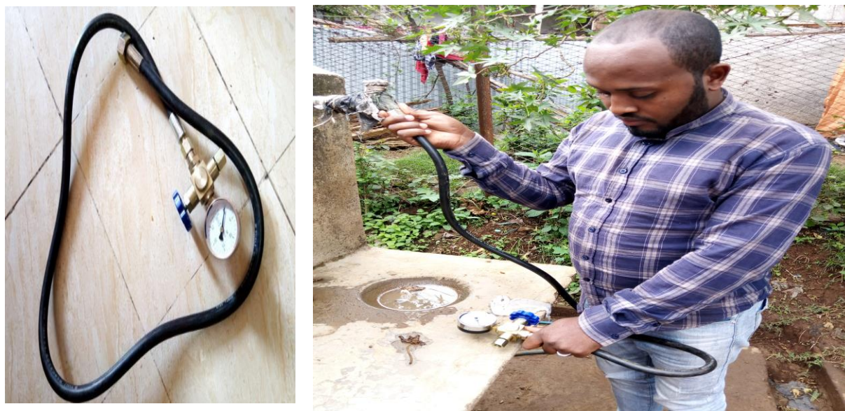
Figure 3-8: Pressure gauge and measuring pressure in the distribution system
