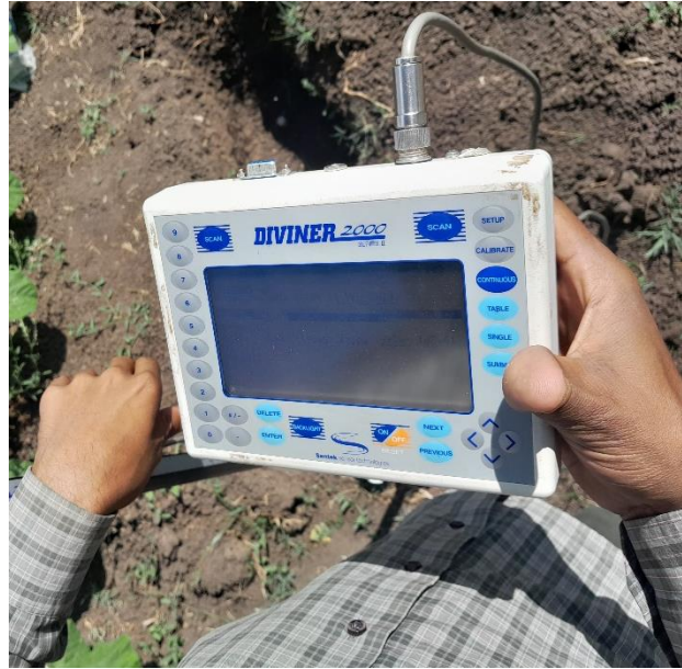
Figure 3-9 Measurement of volumetric water content using Diviner 2000
