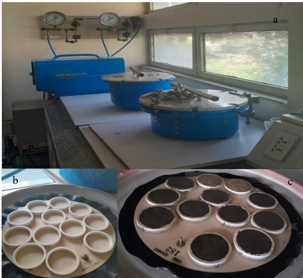
Figure 3-1 a) Pressure plate apparatus b) Ceramic disc c) Soil sample on ceramic plate
