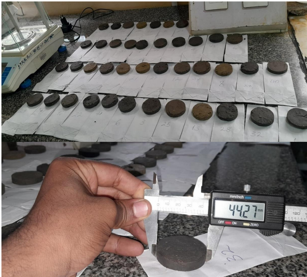
Figure 4-4 Shrinkage curve (SC) determination using Digital Caliper
