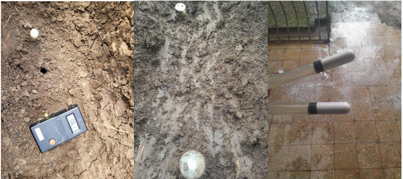
Figure 3-3 Electronic Tensiometer and Probes on Field
