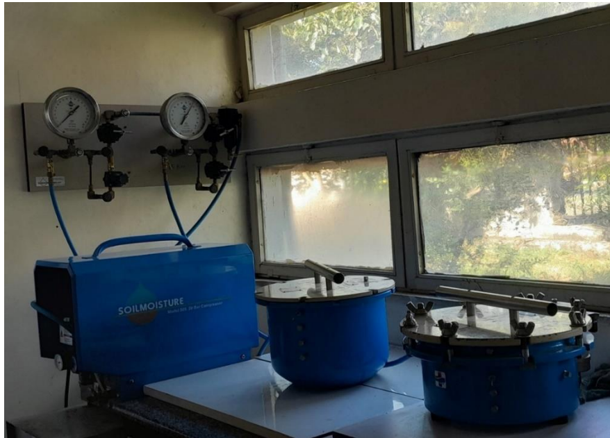
Figure 2-4 Conventional 1500kPa pressure plate extractor (Debre Zeit Institute of Agricultural research)
