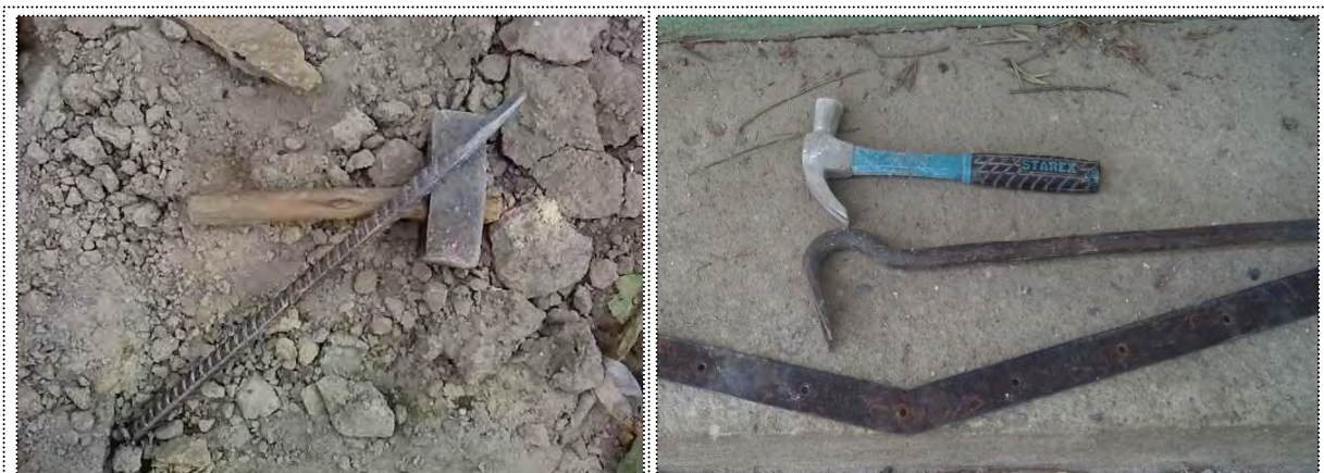
Figure 5.1: Hand held tools used for building dismantling and demolition
