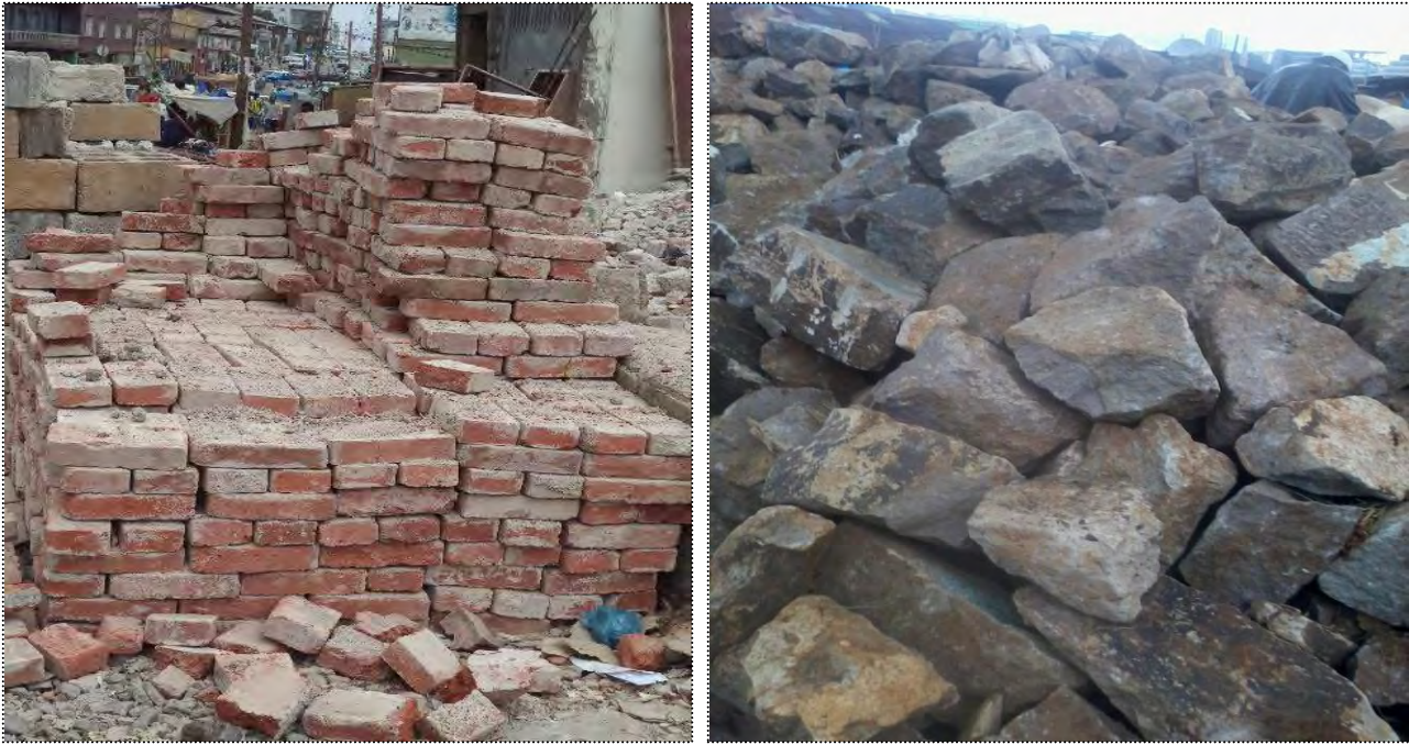
Figure 5.6: Carefully dismantled bricks and dressed stones ( American Gibi )
