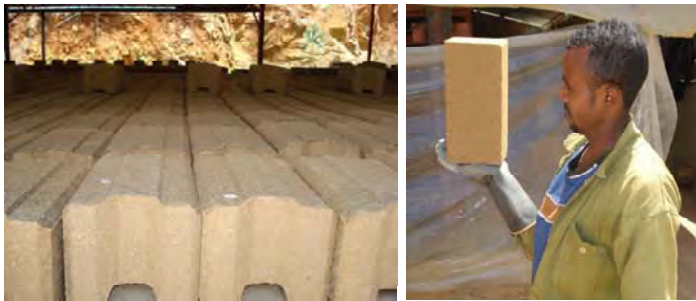
Figure 8-5: a Manually pressed CSSB and Interlocking CSSB at STVC Source: Photo Arash Afkari, Addis Ababa, 2010
