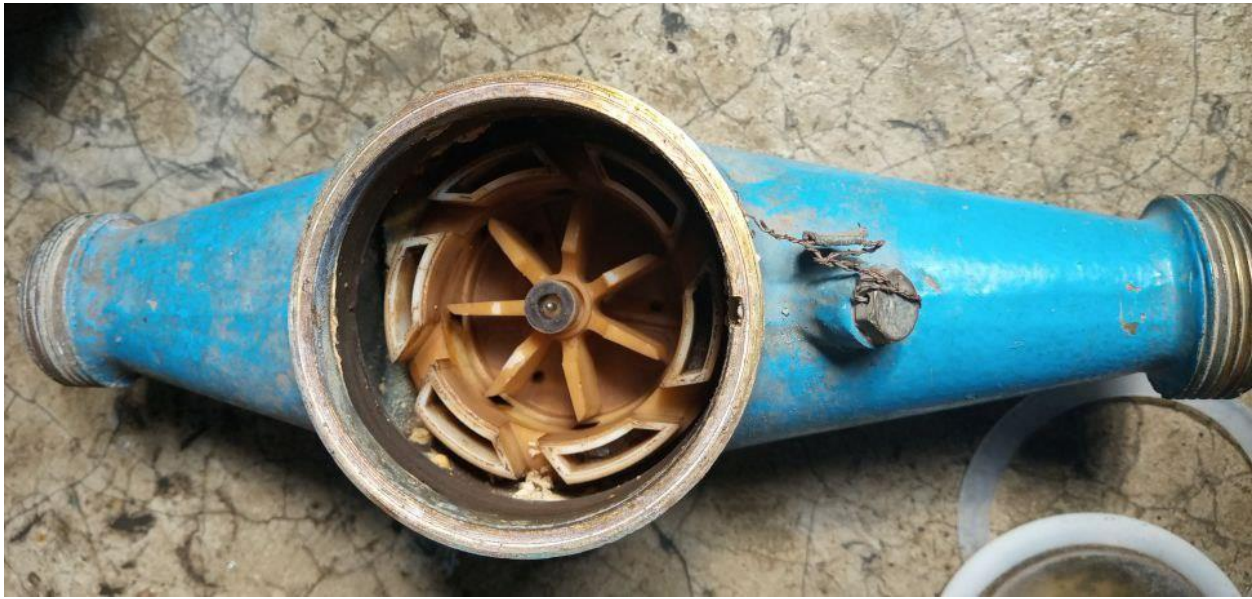
Figure 16 Lime Scale build-up in side of a water meter
