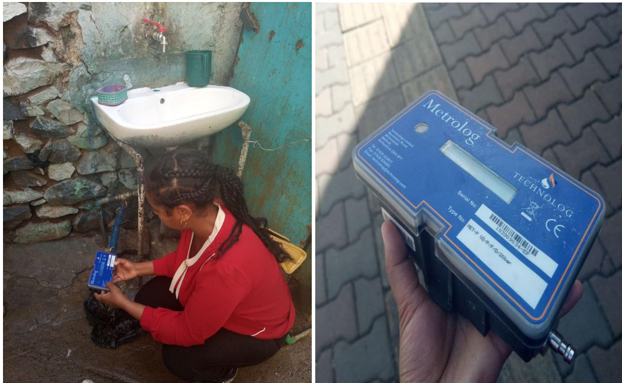
Figure 9 Data logger for pressure measurement
