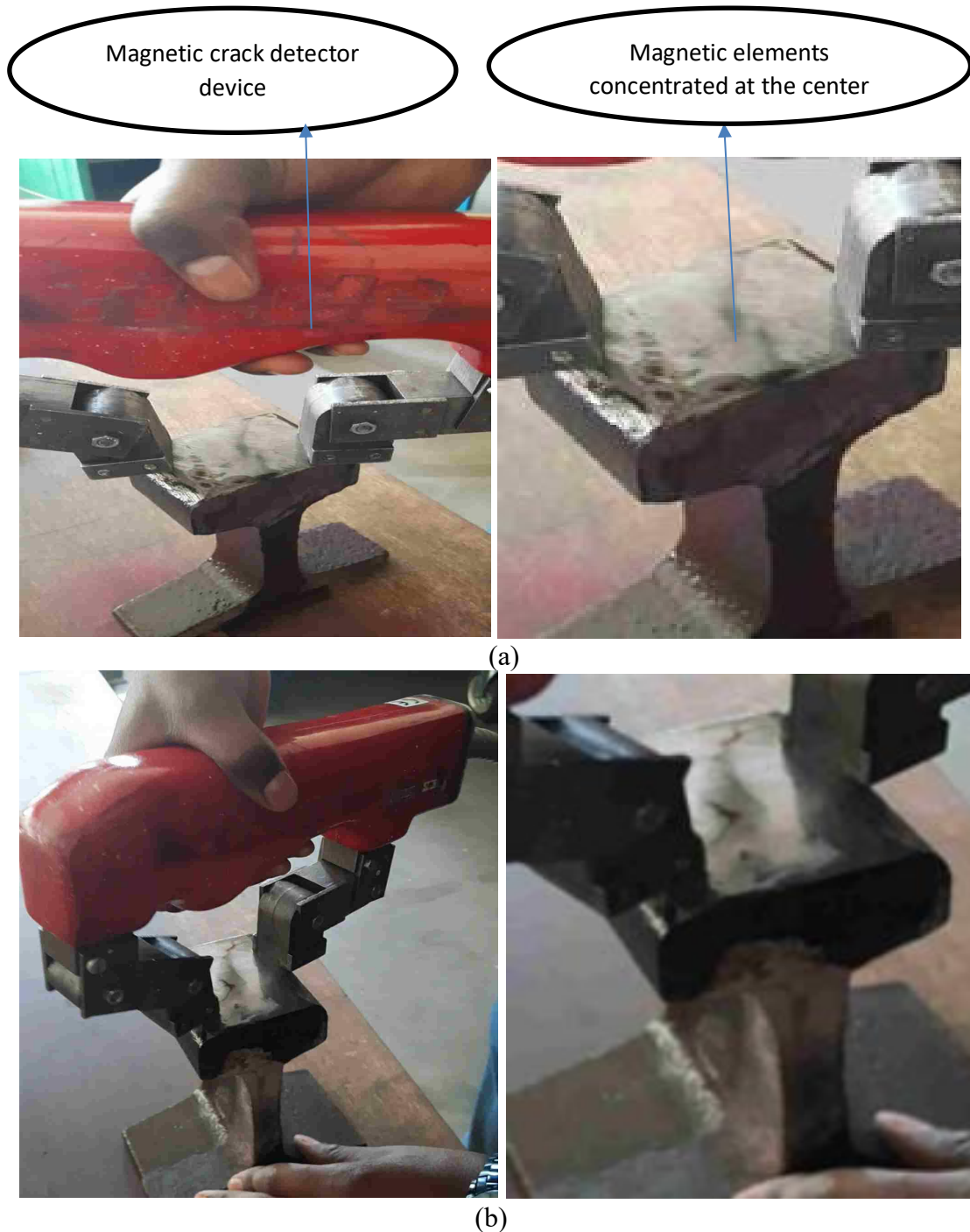
Figure 5-3 Non-destructive crack detection test results using the magnetic field for rail specimens cooled at (a) 2°C/s and (b) 6°C/s respectively
