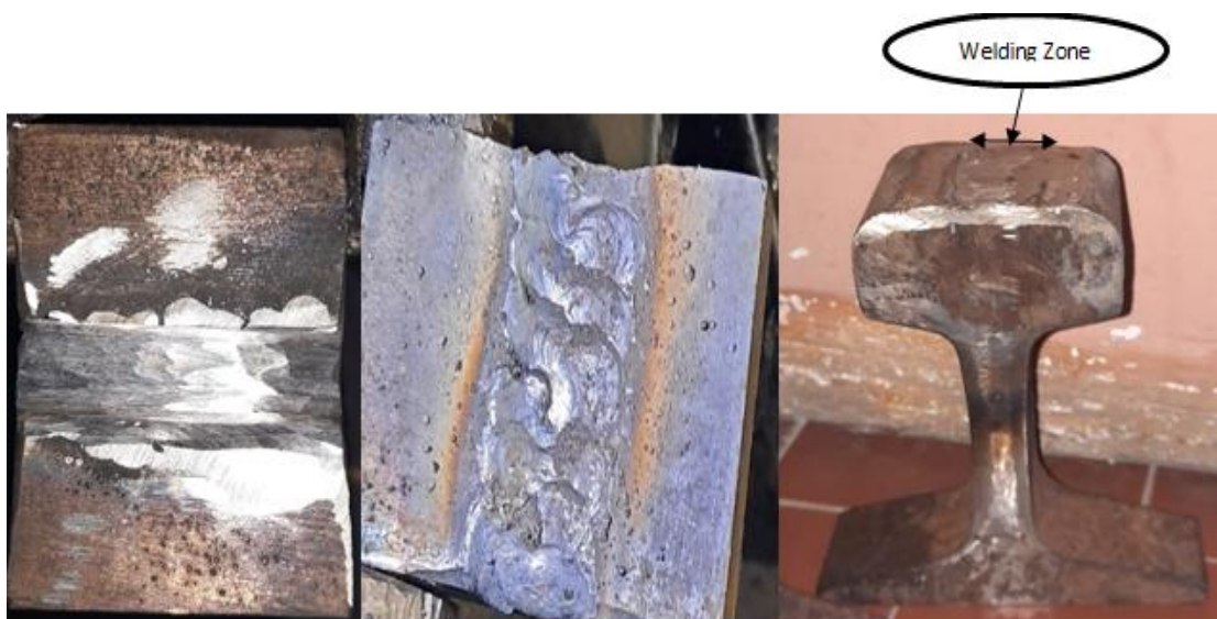
Figure 3- 7 Sample rails artificial damaged and filled by welding
