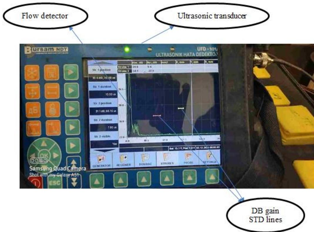
Figure 3- 8 Ultrasonic crack detection device
