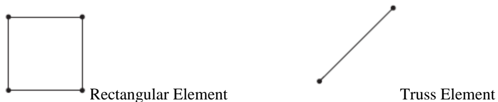
Figure 5.6 : Rectangular and Truss Element Types Used in VecTor2
