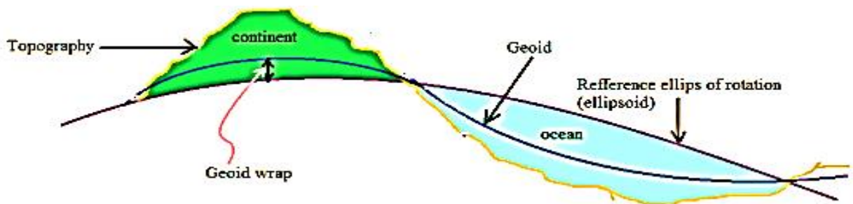
Figure 3.3 geophysical reference surfaces geoid, topography and ellipsoid (after Reynolds, 1997)
