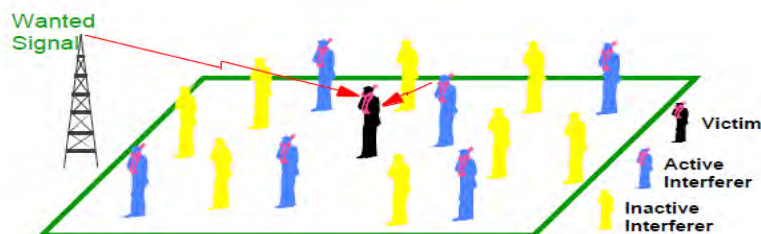
Fig. 2.7 A typical victim and interferer scenario for a SEAMCAT simulation [14].
