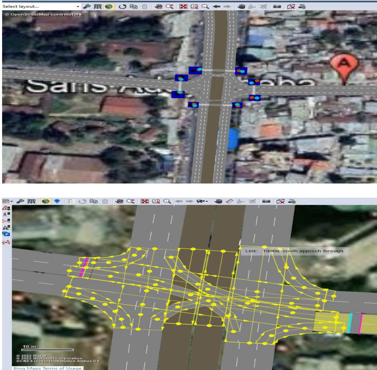
Figure 12. Build background image in VISSIM by Links and Connectors on the study Area
