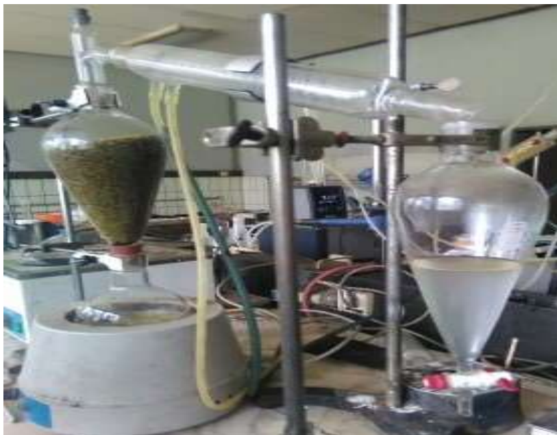
Figure 3.4: Experimental set-up of steam distillation
