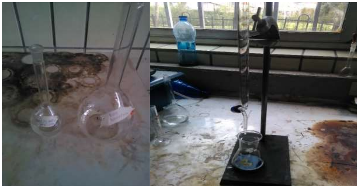
Figure C, 6: Prepared solutions and titrated equipment used for determination of the acid value, saponification value and iodine number
