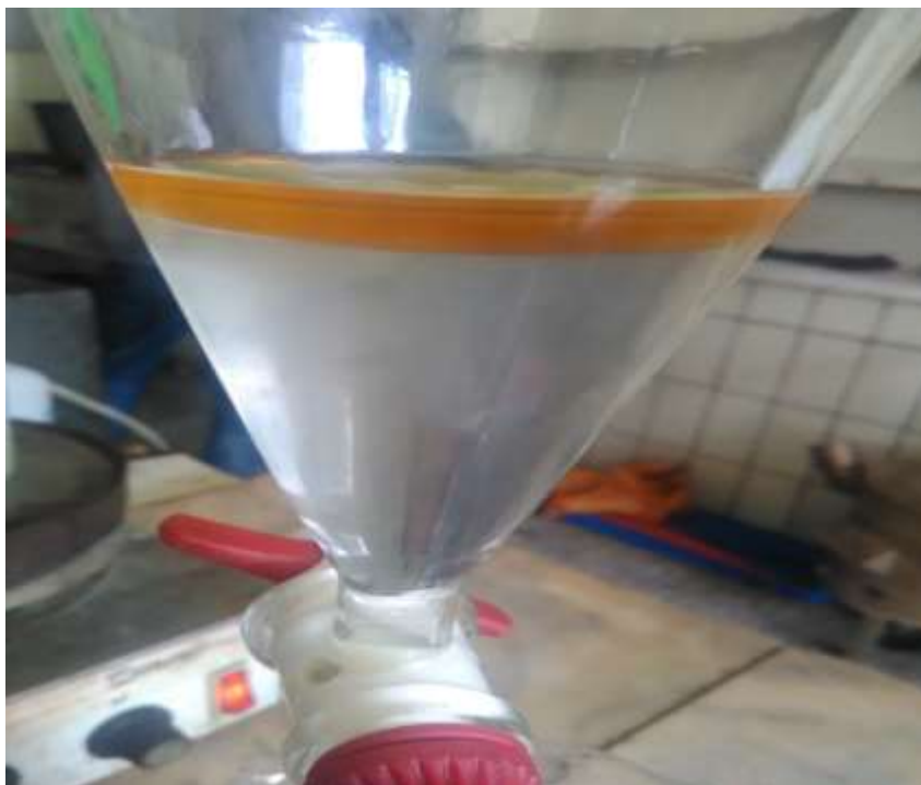
Figure 3.5: separating process of essential oil and water mixture
