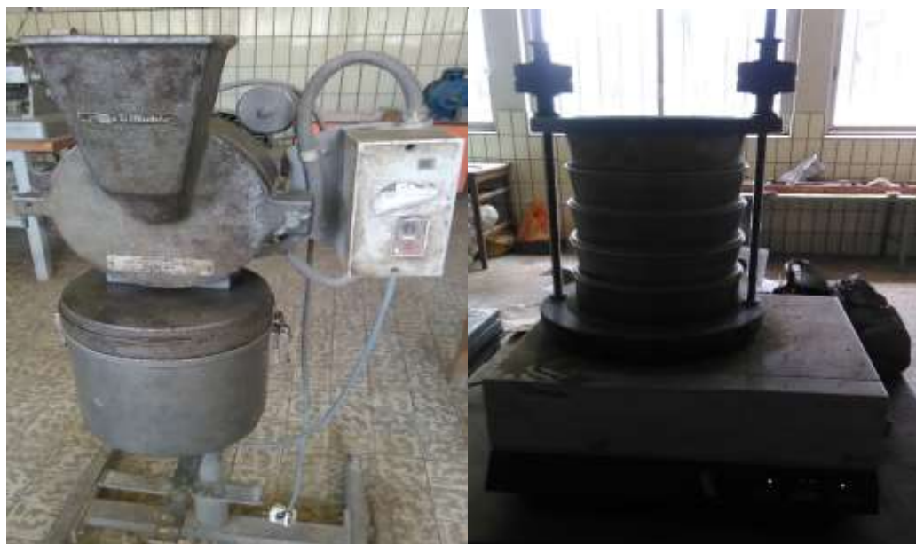
Figure 3.2: Cross beater mill and Sieving analysis
