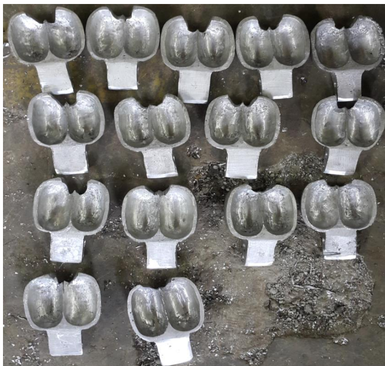
Figure 6.2: Casted Buckets before machining.
