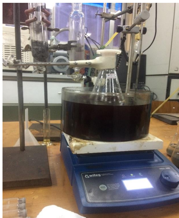
F1: Iron impregnation using MSH-D magnetic stirrer
