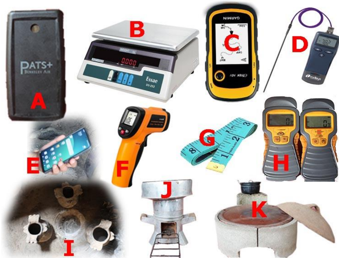
Figure 8: A) Particle and Temperature Sensor (PATS+) B) Electronic weighing balance; capacity of at least 6 kg and accuracy of \pm 1 g C) GPS Tracker D) Thermocouple E) Mobile phone (stop watch) F) IR thermometer G) Measuring tape H) Wood moisture meter; capable of measuring 6-40% humidity (optional) I) Choche stove J) Tikikil stove K) Mirt stove (Pictures By: Dawit.T)
