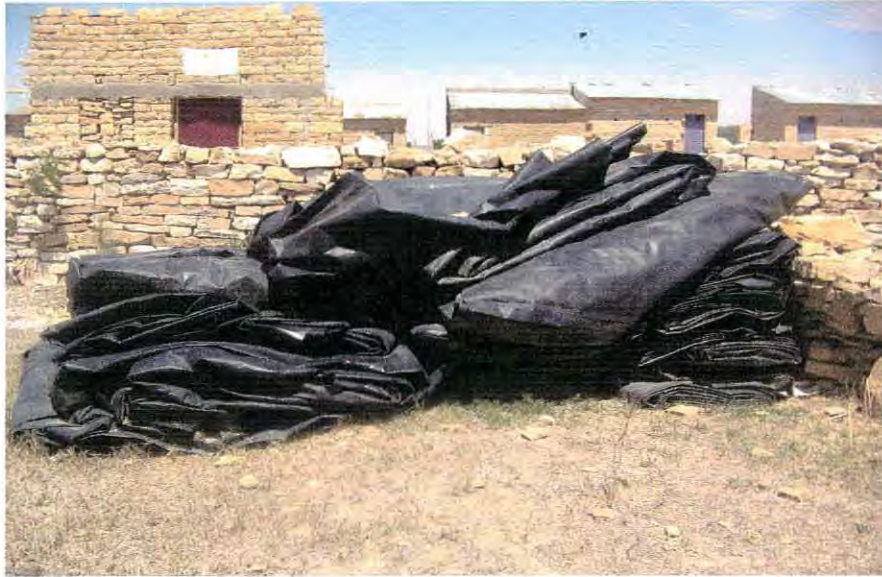
Plate 4.4: Lack of proper storage damaged the plastic linings
