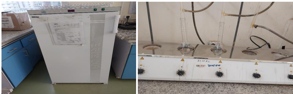
BOD Incubator & COD analysis of wastewater respectively
