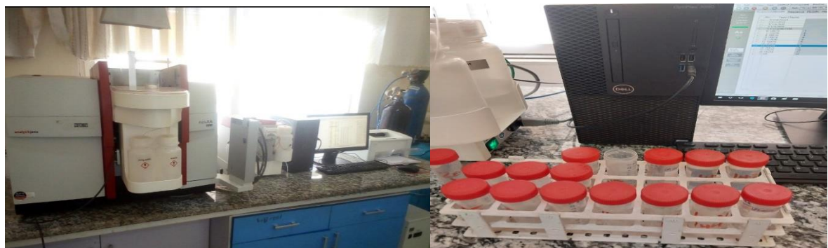
Graphite Furnace Atomic Absorption Spectroscopy for reading of Lead metal ion for untreated wastewater sample & wastewater treated by MASA adsorbent
