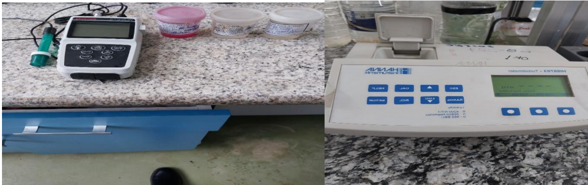
pH & Turbidity meter used for test pH of wastewater and turbidity of wastewater respectively.
