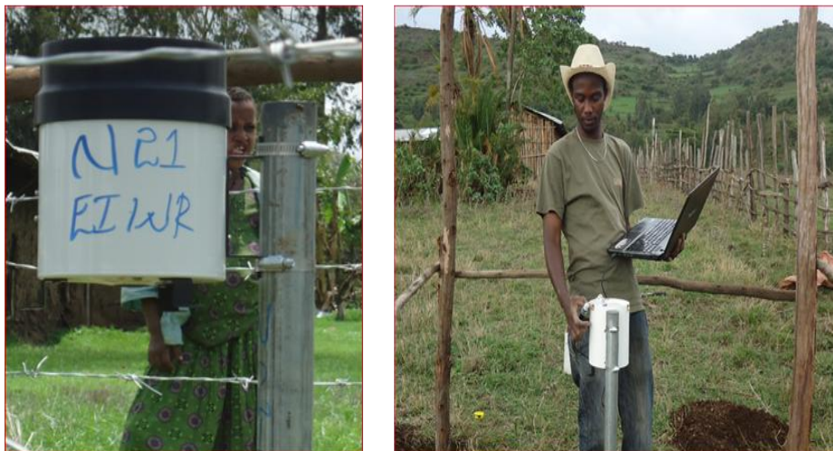
Fig. 4.2 A photographic view of Tipping Bucket rain gauge electronic recorder during its installation and data collection.
