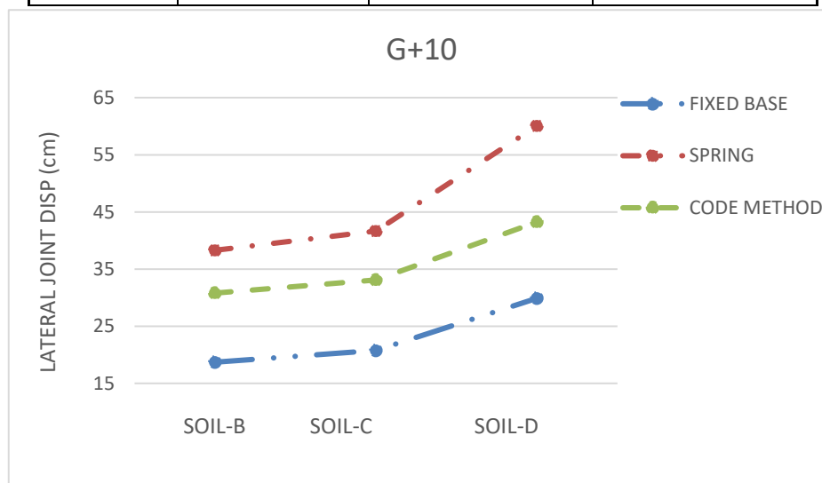
Figure 4-16: Lateral joint displacement at roof level of G+10
