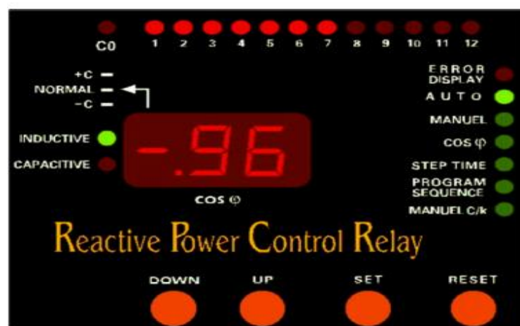
Figure 3. 12: Automatic power factor control relay [14]
