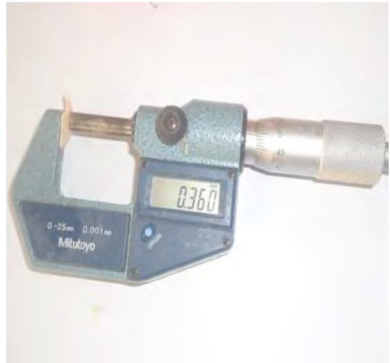
Annex 3: Measuring eggshell thickness using digital Caliper
