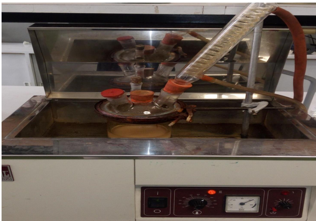
Figure 2.1: Three neck glass chemical reactor vessel over thermostated water bath (GFL ® , D3006, Germany) for carboxymethylation of Dioscorea bulbifera starch (Picture taken by Meseret A.).
