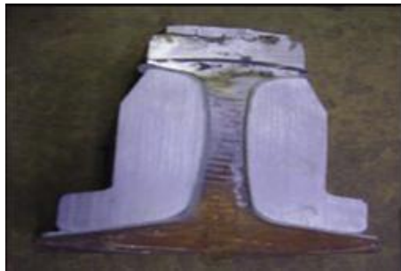
(g) Chipping at rail end and gage corner
