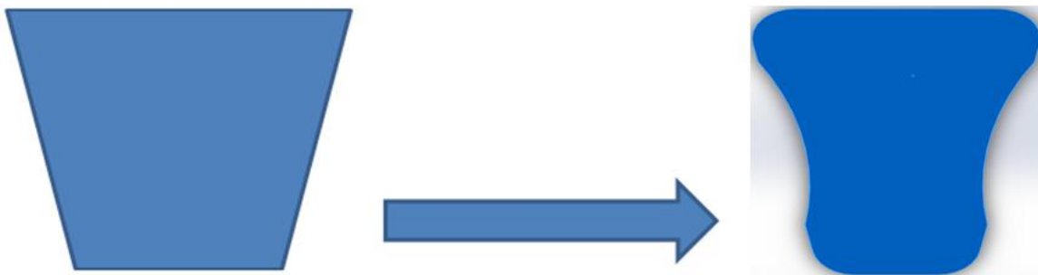
Figure 3-4: cross section of model 2 crane hook
