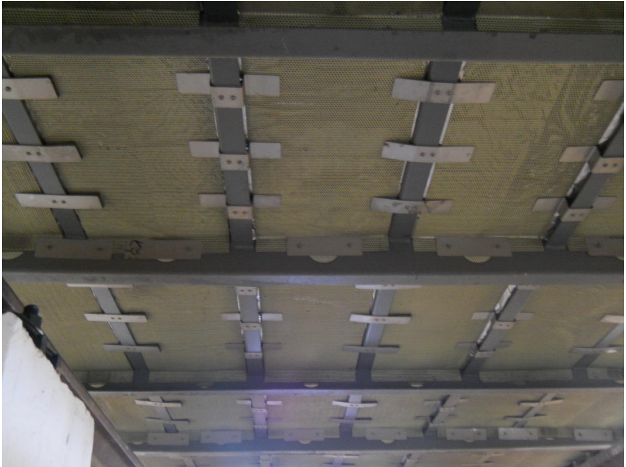
Fig 3.1 Under frame structure on the train Mc low floor area
