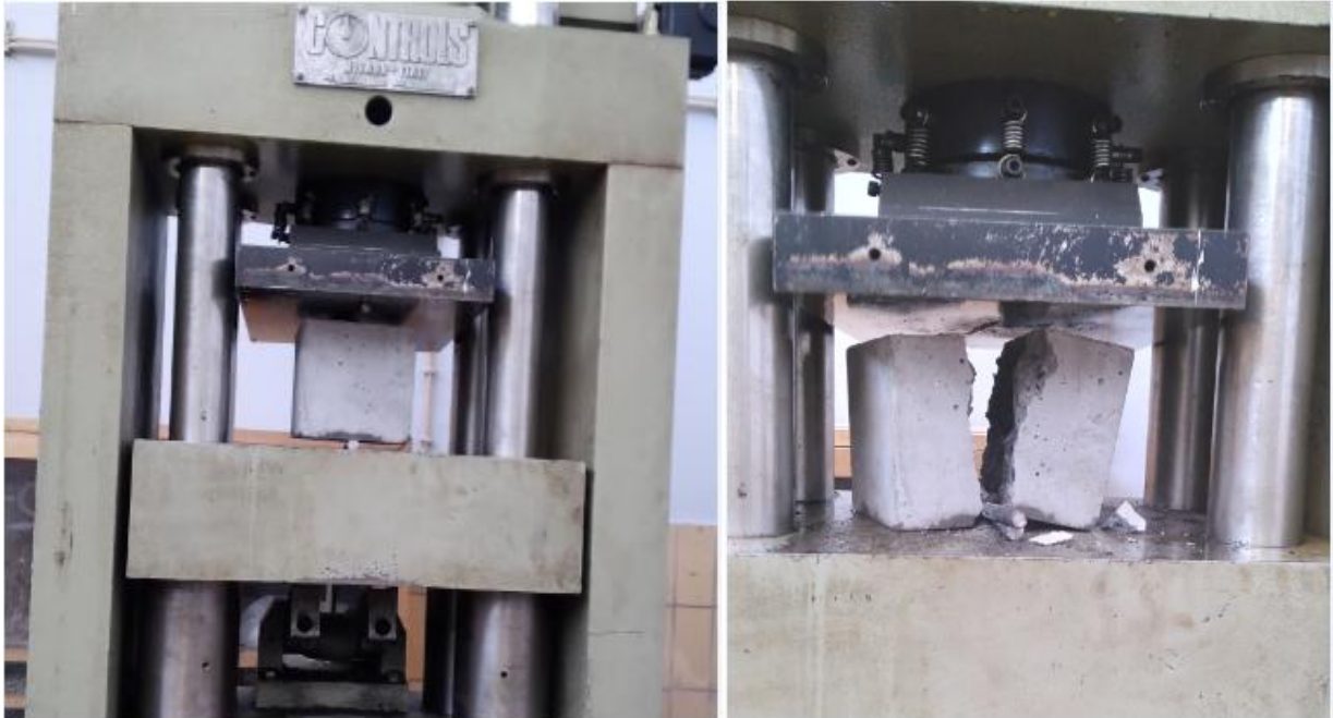
Figure 4. 6 concrete cube passing water penetration test when ready to be split (left) and after it was split (right).
