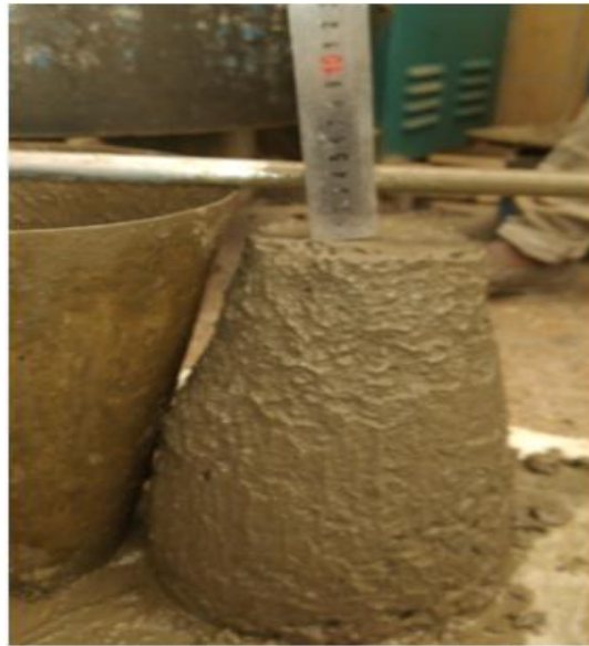
Figure 3. 9 Measuring Slump of Fresh Concrete
