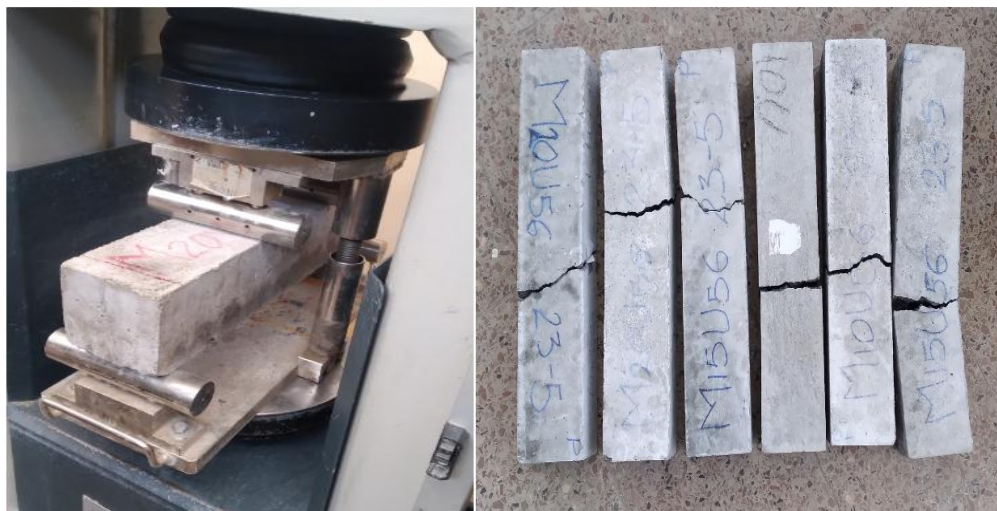
Figure 4. 3 (a) Test Set up of flexural Strength Test (b) Test Specimen after Failure
