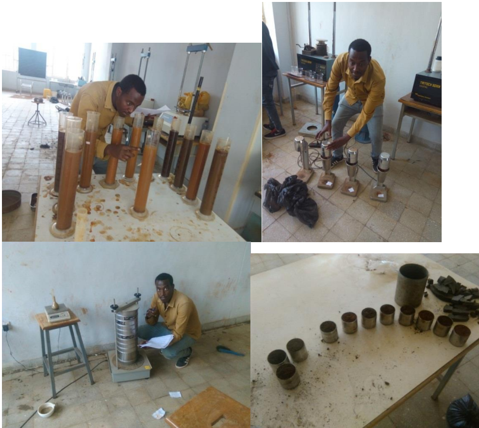
Annex figure 2: Soil hydrometry analysis in laboratory recording reading (a), shaking for 10min (b), soil sieve analysis (c), and soil moisture content analysis in laboratory (d)
