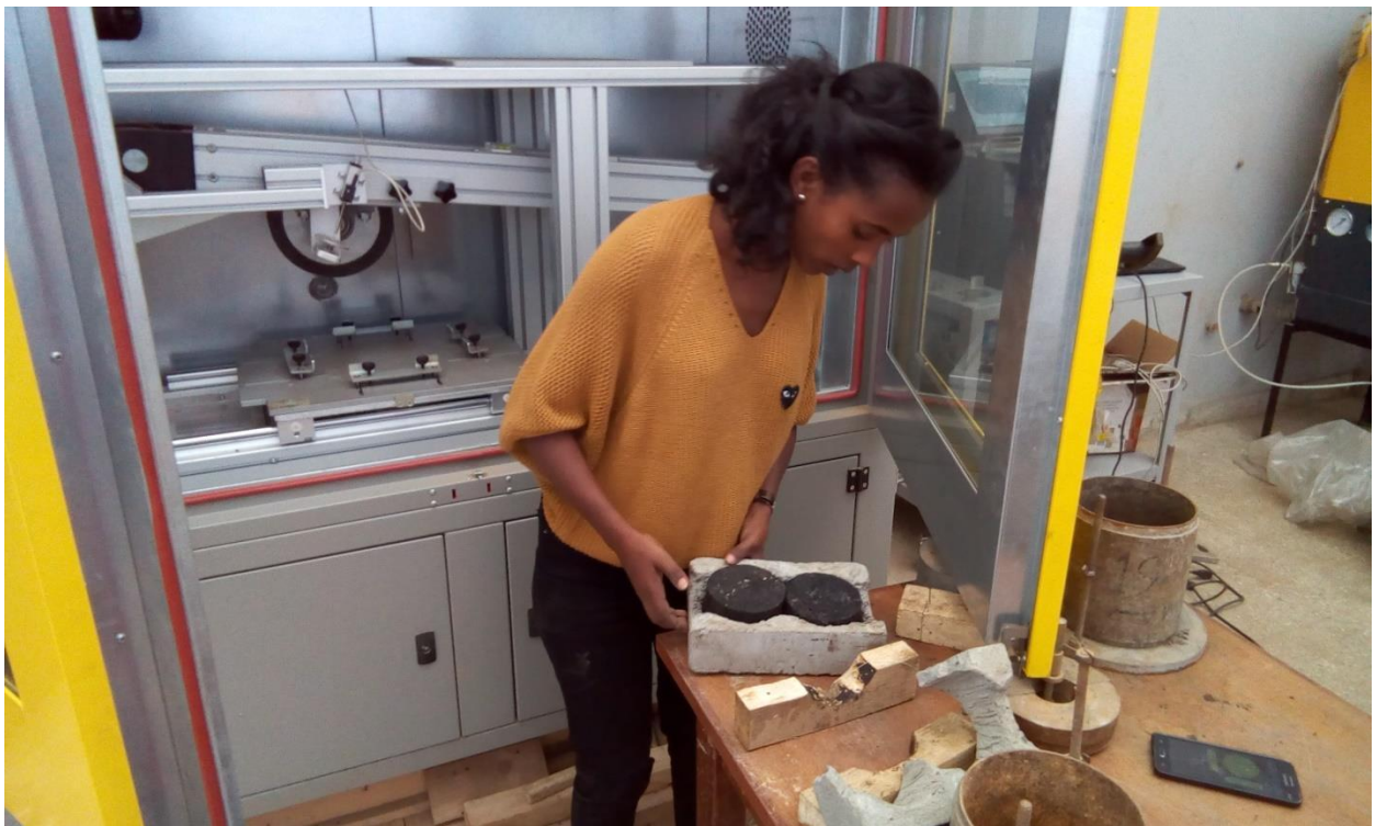
Caption 9: preparing specimens for Dyna track wheel load tester
