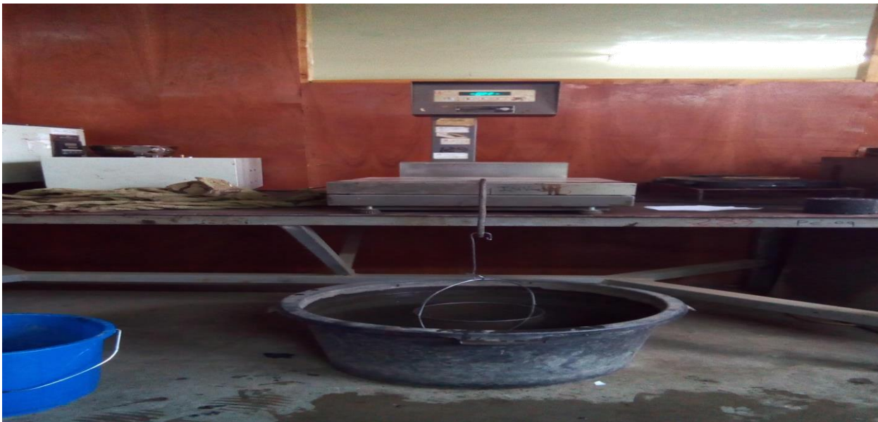
Caption 7: Weighting specimen in water
