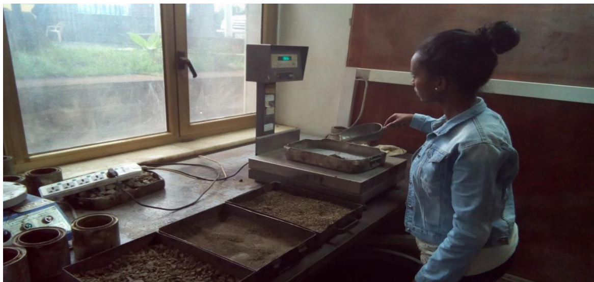
Caption 2: Weighting of the sample aggregates
