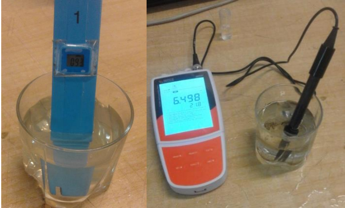
Turbidity, PH, and Conductivity testing
