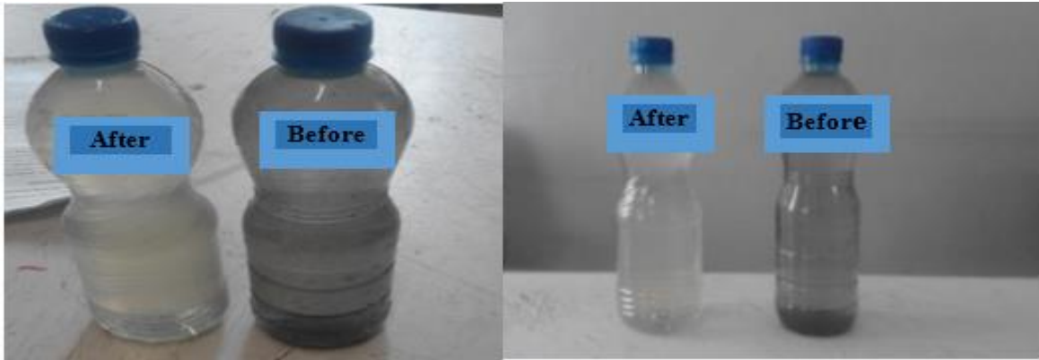
Figure 5.6: Turbidity before and after entering of the Bio-retention system
