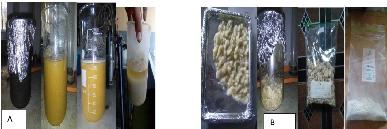
A) samples from extractives removal, delignification and hemicellulose removal B) extracted micro-cellulose: drying and packaging
