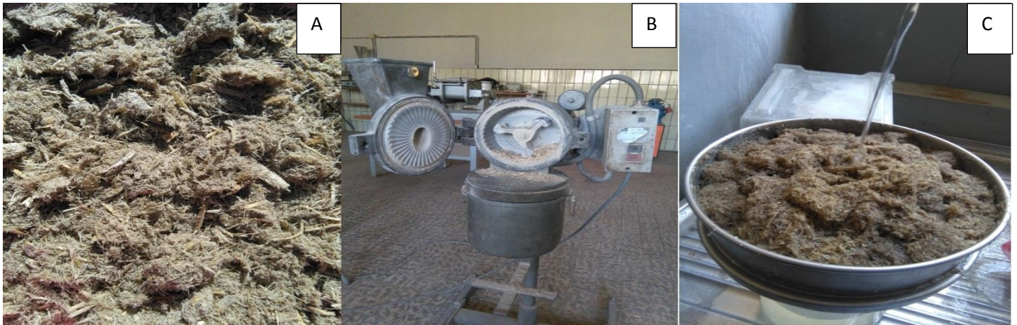
A) bagasse as it was brought from wonji showa sugar factory B) size reducing unit operation c) size reduced bagasse under washing
