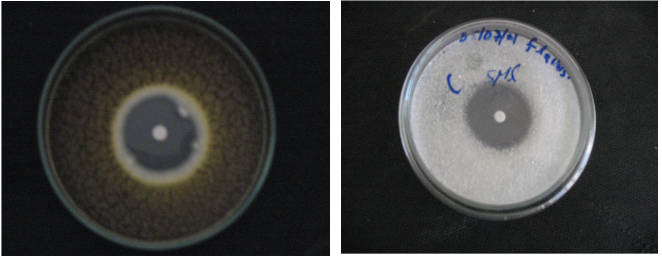
Fig.4. Growth inhibition zone diameter on Aspergillus niger and Aspergillus flavus by cinnamon essential oil
