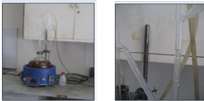
Fig.2. Hydro-distillation apparatus set up
