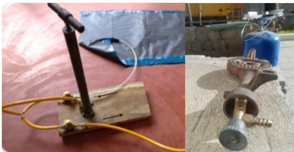
Figure 56 Configuration of hand pump used to bottle biogas in the cylinder
