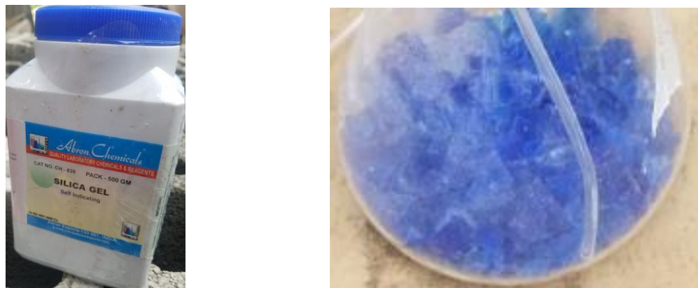
Figure 36 Removal of water vapor from Biogas
