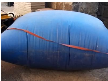
Figure 42 Biogas bag used as biogas storage option
