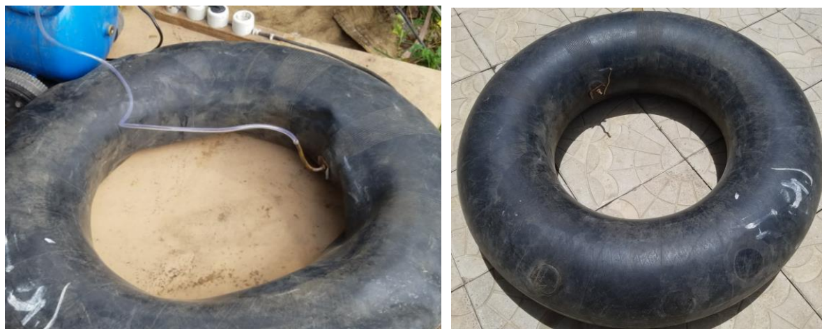
Figure 44 Tire Inner Tube before and after biogas storage
