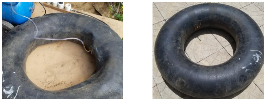
Figure 41 Tire inner tube used for biogas storage option
