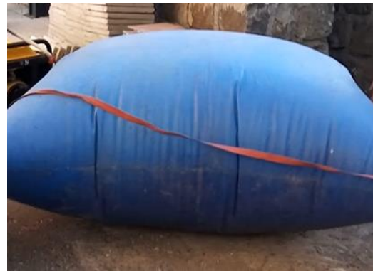
Figure 52 Biogas compressed and stored into ballon and biogas bag
