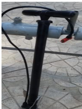
Figure 55 Hand (cycle) pump used to bottle gas in to a cylinder
