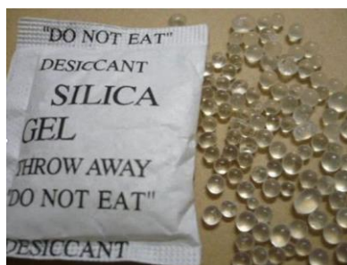
Figure 17 Removal of water vapor from Biogas [36]
