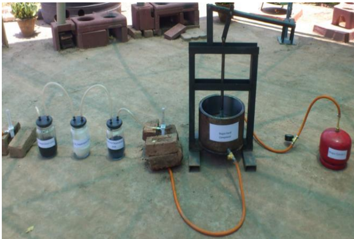
Figure 7 Typical arrangement of biogas compression and bottling process [31, 41]
