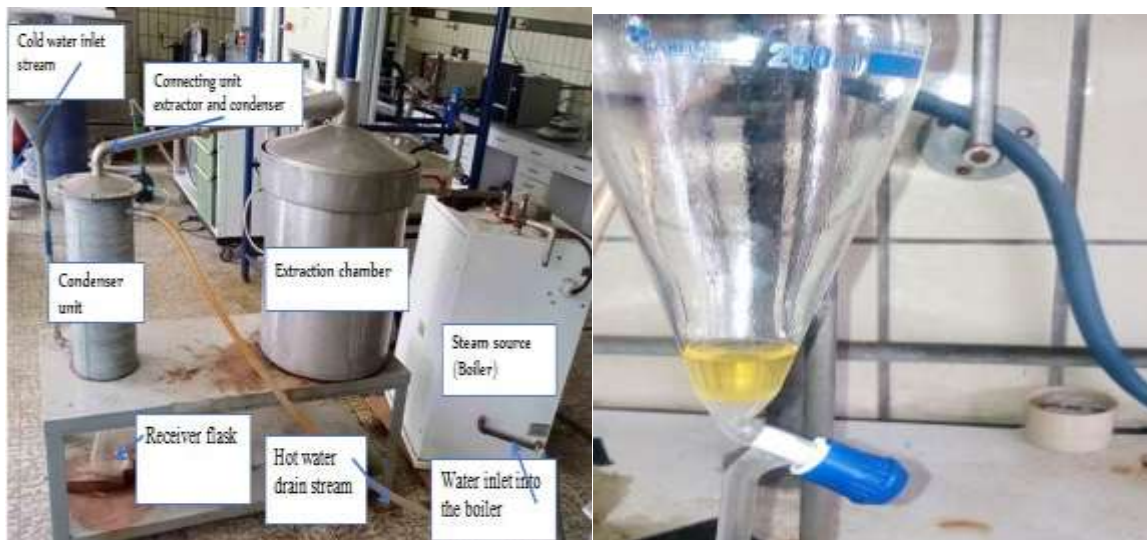
B2: Lemongrass essential oil extraction by steam distillation setup
