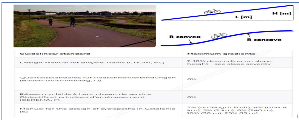
Figure 9 shows gradients and recommended slope (source: Design manual for cycle traffic .crow NL)
