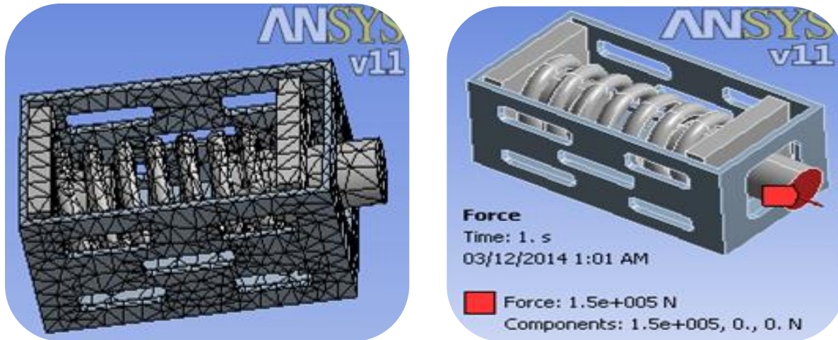
Figure -4.14. Mesh and boundary conditions for compressive load for coupler
