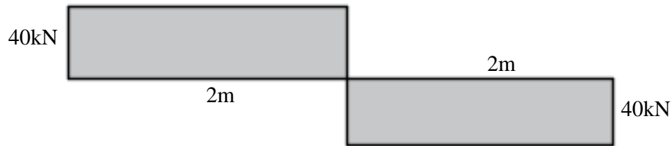
Figure 4.3 Shear force diagram of beam 2
