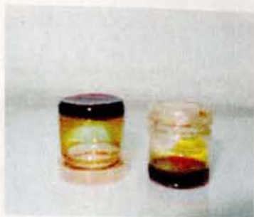
Figure 3. 5: Polymer gel electrolyte composed of polymer PVP, EMIm-I, NaI, and I_2 as quasi-solid state electrolyte.
