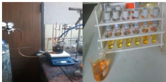
Figure 3-9: a) Decarboxylation process setup at 120 °C, and; b) Dimethyl benzene samples.
